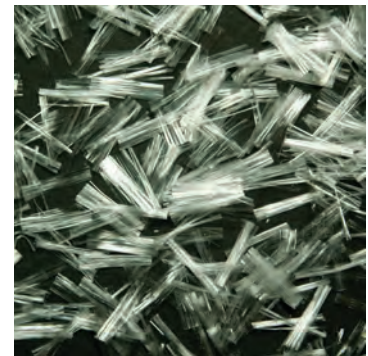
Figure 2: Fibrillated fibers (Grace Fibers shown)
