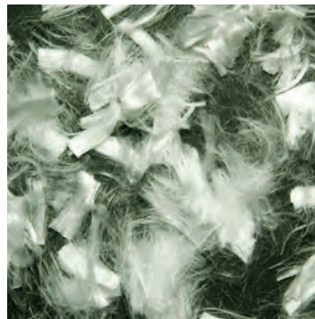
Figure 1: Monofilament fibers (Grace MicroFibers shown)
