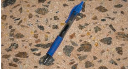
Photo B: In areas where the surface was polished down to expose the coarse aggregate, the fibers were not visible at all.
