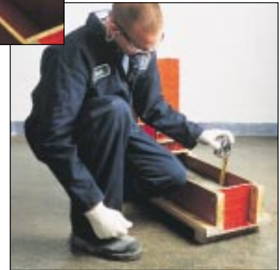
L Box Test to measure flow and blocking resistance of mix
