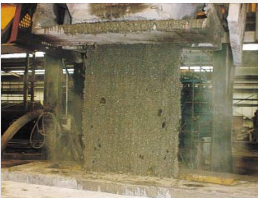
Self Consolidating Concrete in precast production fills formwork without segregation or blocking.
