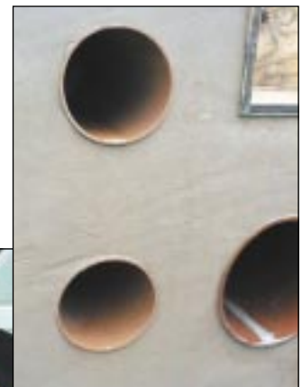
SCC flows and compacts around obstacles and reinforcement to give complete consolidation.
