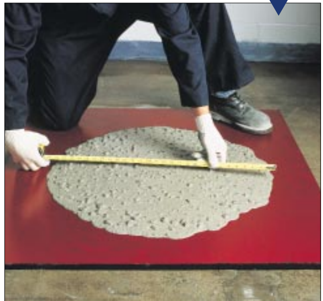
Slump Flow Test to measure slump diameter
